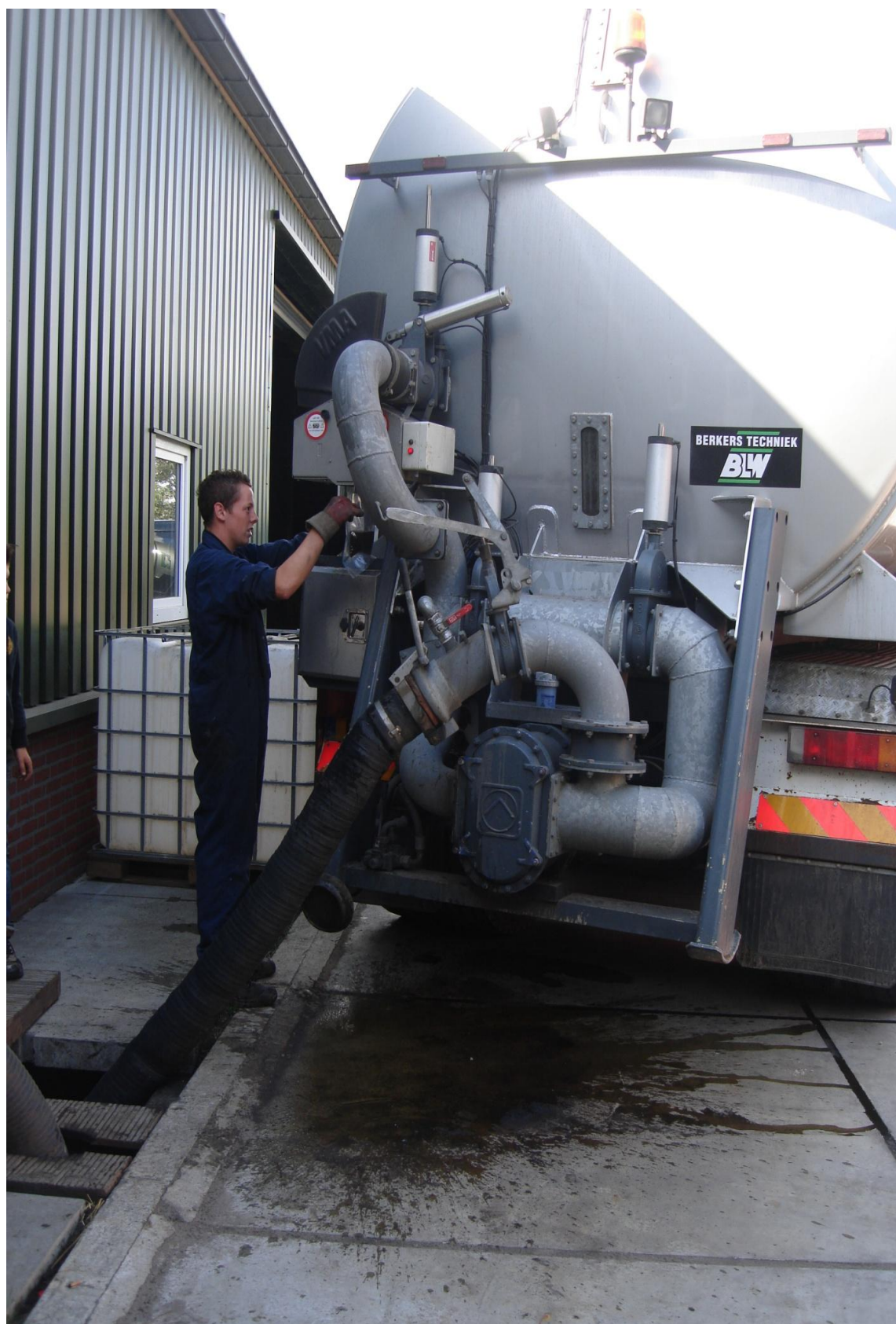
Picture C.10: The nitrogen rich fraction is kept in covered storage tanks, and here loaded by a truck. A representative sample is taken during loading.
