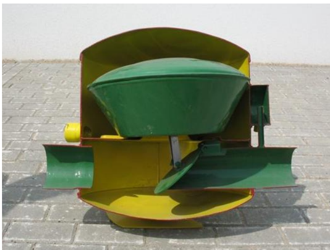
REGULATION UNIT FOR ON/OFF DRAINAGE DEVELOPED IN FORMER EASTERN GERMANY IN 1989.
