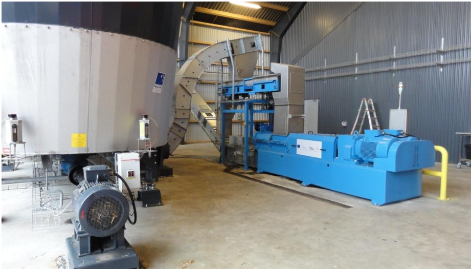
THE BIO-MIXER TO THE LEFT AUTOMATICALLY FEEDS THE TORN APART BIOMASS INTO THE EXTRUDER FROM WHERE IT IS LED TO THE DIGESTER TANK.
