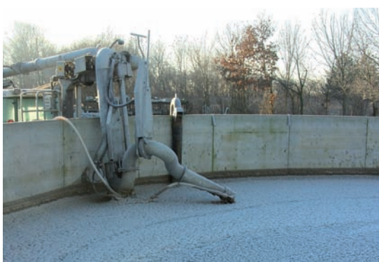
Acidification in the slurry storage is done in connection with agitating just before field application.
