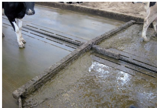
Wire dragged scraper used on a solid, drained floor in a dairy cow unit.
