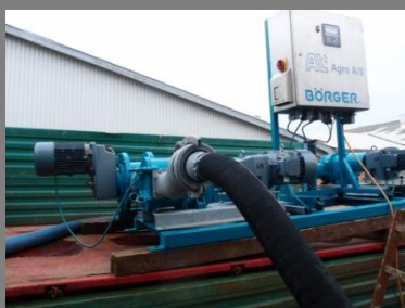
Quick slurry separation, Börger AL-2 separator. Photos 2011 by Environmental consultant Elisabeth Falk, The Bornholm Advisory Service.
