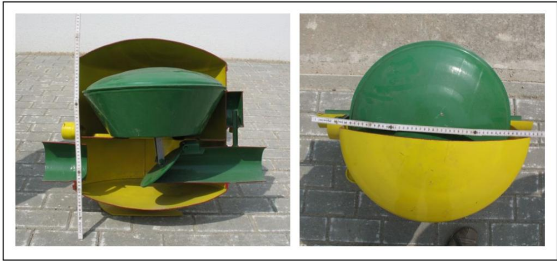
Figure 2: Drainage regulation device (Source: Dr. Jörg Steidl, Leibniz Centre for Agricultural Landscape Research (ZALF), Institute of Landscape Hydrology)
