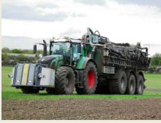
Slurry spreading tanker mounted with BioCover's SyreN technology for slurry acidification during field spreading.
