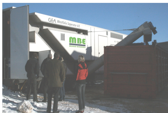
Mobile decanter centrifuge with use of flocculation
