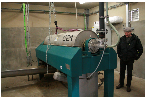
Decanter centrifuge for post separation
