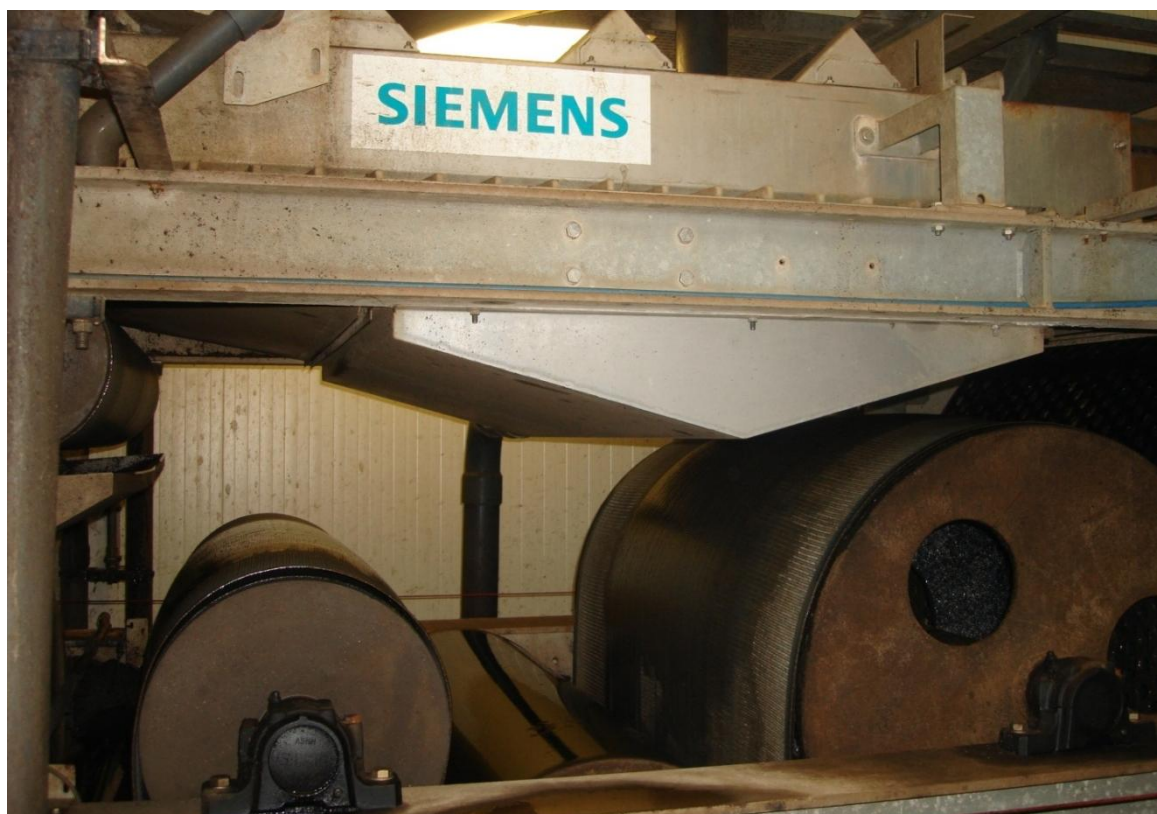
Picture 4: Separation with filter belt press, after treatment with an additive and a polymer.
