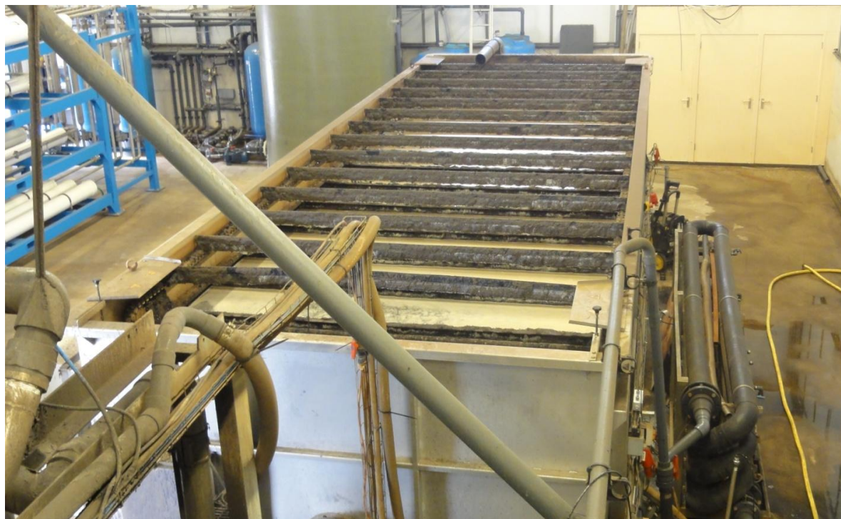
Picture 7: Scrapers remove the flotation sludge from the flotation unit.
