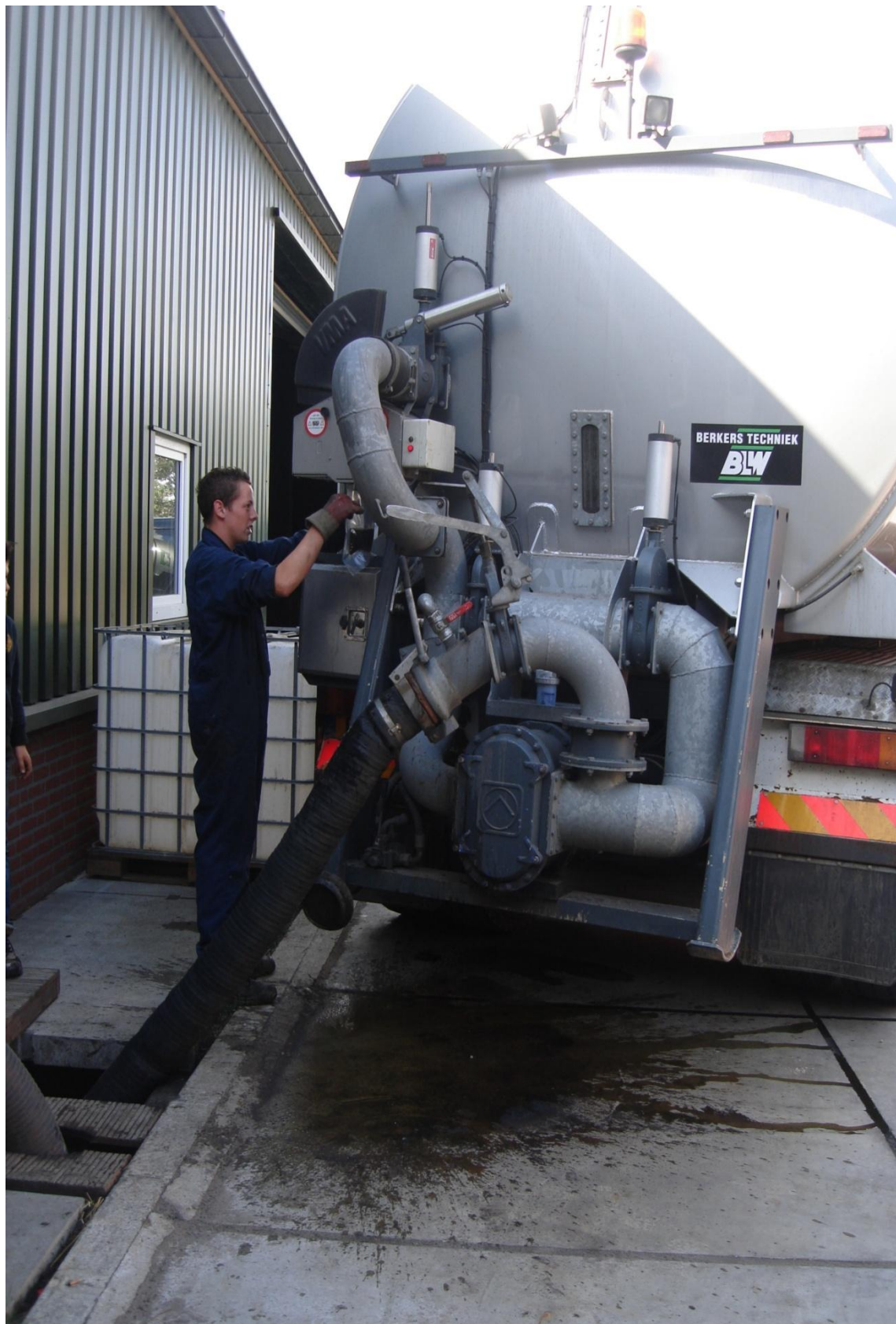
Picture 10: The nitrogen rich fraction is kept in covered storage tanks, and here loaded by a truck. A representative sample is taken during loading.
